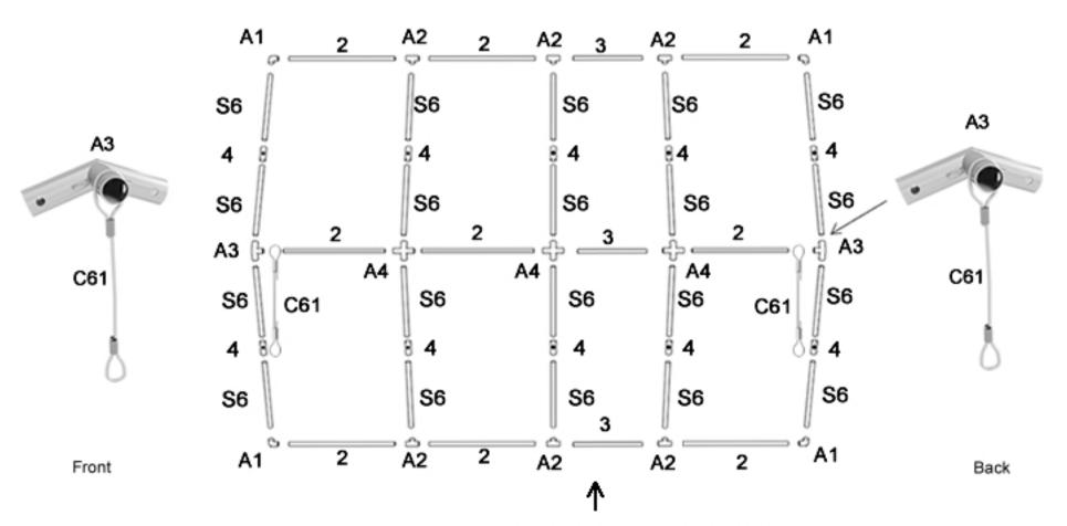
The extension tube (3) should be located in the third section.
