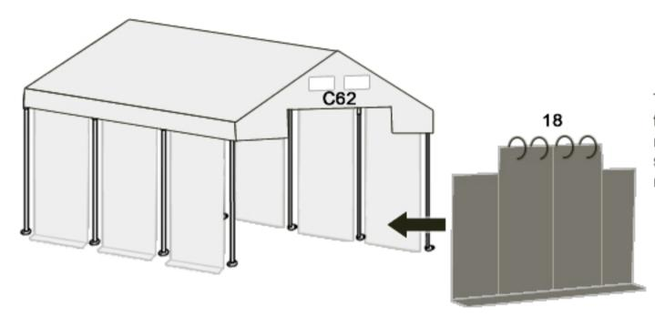
The upper part of the entrance using the metal brackets (18) to the vertical rope (C62). The sides of the entrance should be mounted using the elastic rubber with the ball.
