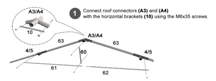
Connect the brackets (61) and (62) using the M6x35 screws. Connect the obtained construction to the 2 lower part of connectors (4 or 5).
