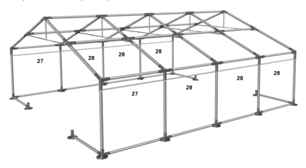
Pass the pipe number 30 through the cover's stitching. Connect pipe (30) with tube (27 or 28), using strings with clips. For tents with the 1m extension, instead of using tube (28) use tube (29). Instead of using tube (30) use tube (31).
