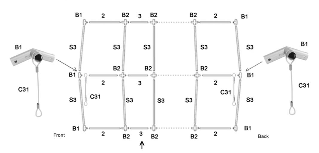
The extension tube (3) should be located in the second section.
