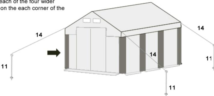
Fix the roof pulls on the corners of the tent using the **(14)** and **(11)** parts. All the lines should be tight.
