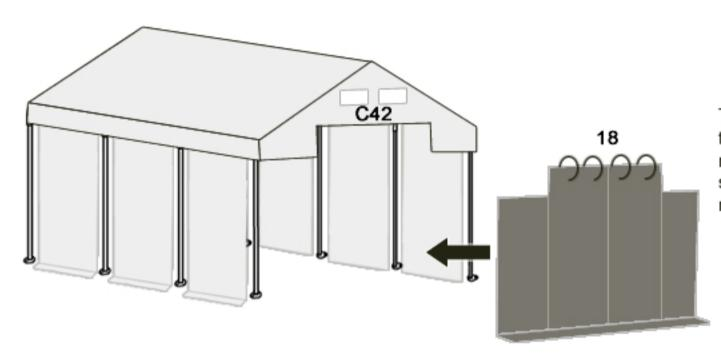
The upper part of the entrance using the metal brackets (18) to the vertical rope (C42). The sides of the entrance should be mounted using the elastic rubber with the ball.
