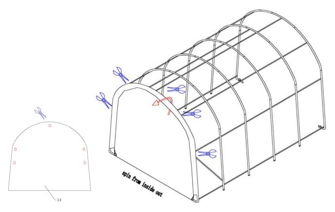
1. Put on the Front Door cover (part No.14) from the inside of the door frame to the outside and find the suitable holes to pass throw all the tubes. Fix them using Rope inside of the door cover and tie it on the bottom of the door frame. Then put on the back door cover like it.
