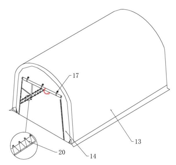
3. Knit the Roof Cover and the Lowest Horizontal Connecting Tubes by using the Rope (part No. 20).
