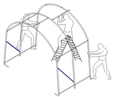
2. By turn, connect the other group arches by using Male Horizontal Connecting Tube (part No.5) and Bolt M8\*80mm (part No.15) Please make the Horizontal Connecting Tube under the arch frame, the roof cover could be supported beautifully.
