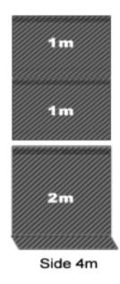
Assembled panels are ready to be mounted using the velcros on the roof. In order to fix the panels on the sides the elastic rubber with the ball should be used.
