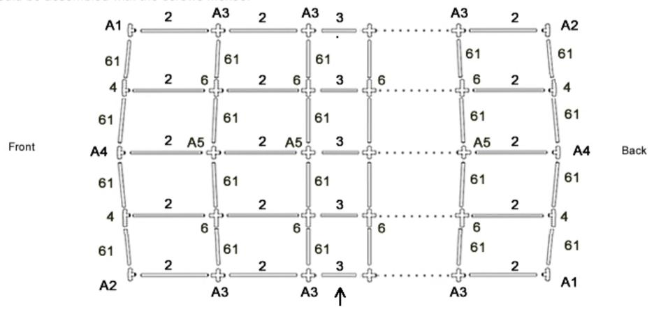
The extension tube should be located in the third section.
