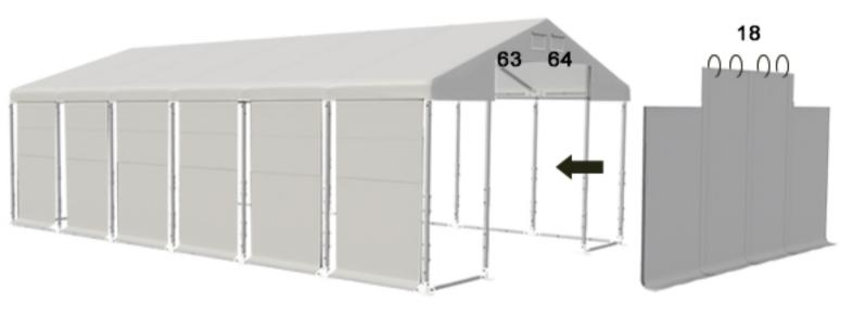
Mount the entrances on the both sides of the tent. Use metal loops (18) to mount the upper part of the entrance to the vertical tube (63 and 64 put together). Sides of the entrance fix using the elastic rubbers with the balls.
