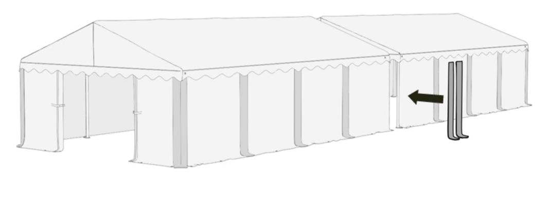
Mount connecting gutter to the roof tarpaulin with the valcros and balls with rubber.
