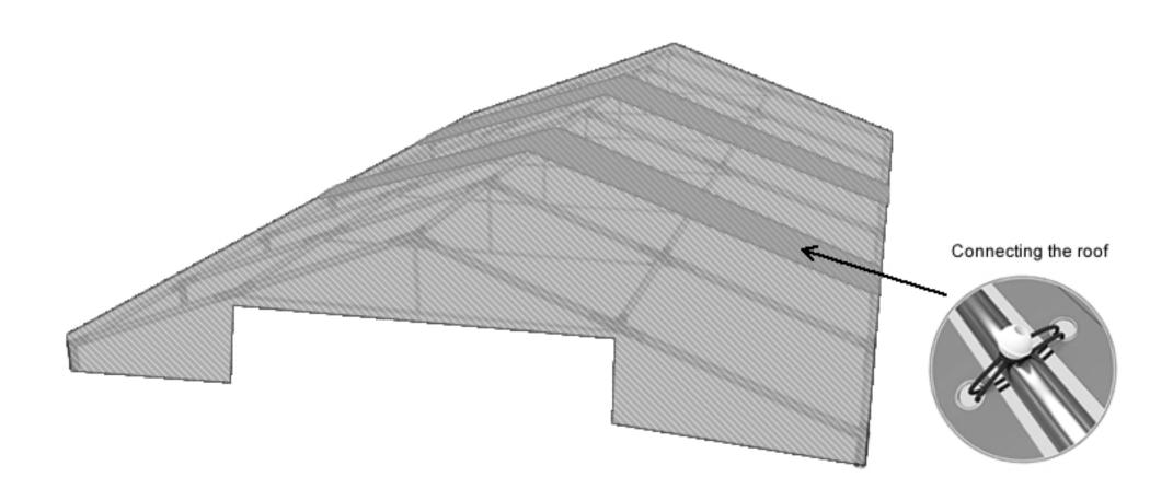
Pipes to attach the cover (27 and 28) should be installed on the inside of the tent.
