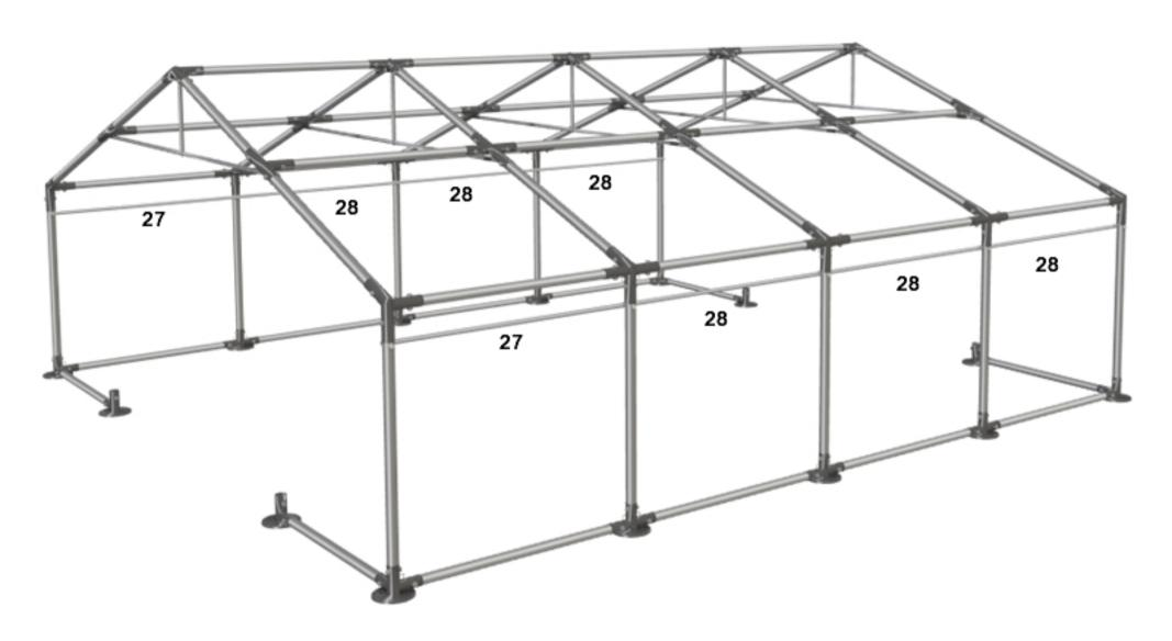
Pass the pipe number 30 through the cover's stitching. Connect tube (30) with tube (27 or 28), using strings with clips. For tents with the 1m extension, instead of using tube (28) use tube (29). Instead of using tube (30) use tube (31).
